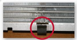
Installation damage/improper installation Damage resulting from improper or incomplete installation or abuse by the installer isn't covered by warranty. This radiator was damaged when the installer clipped the tube while installing the fan shroud clip. Always use caution during installation to avoid radiator damage.
